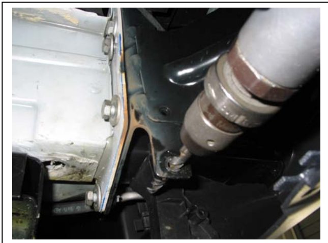
Figure 5 – Driver's side shown enlarging existing hole M10 x 40 x 1.5 bolts
